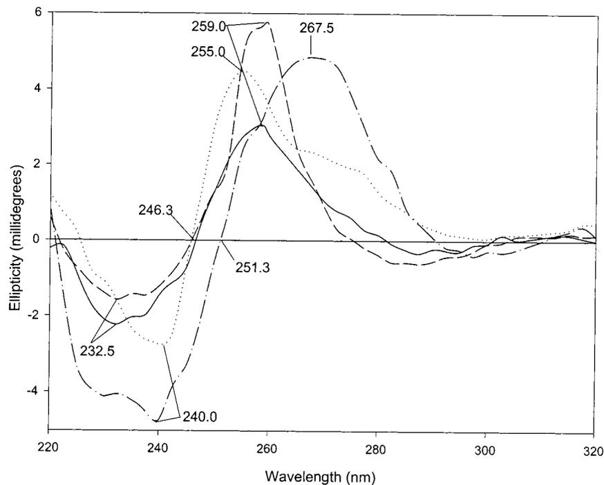
**Figure 5.** CD spectra of racemic ( $\text{Ru}^{2+}$ -DNA)·DNA duplexes as a function of wavelength (nm): **10·13** (—), **11·13** (···), **12·13** (---). CD spectra of nonmodified DNA·DNA duplex **9·13** (-·-) is shown for comparison.
