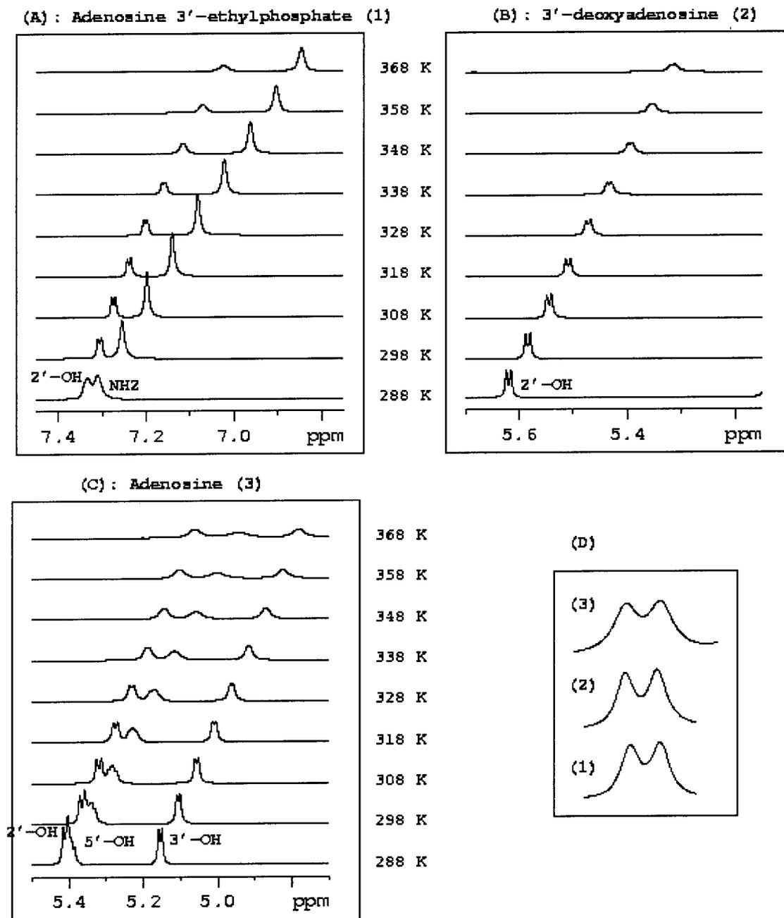
**Figure 4.** Panels A–C show the temperature-dependent (over the range of 288–368 K) hydroxyl resonances for adenosine 3'-ethyl phosphate (**1**), 3'-deoxyadenosine (**2**), and adenosine (**3**), respectively, in DMSO- $d_6$ . Panel D shows the comparison of  $^3J_{\text{H}2',\text{OH}}$  for **1–3** (4.2 Hz for **1**, 4.3 Hz for **2**, and 6.0 Hz for **3**) at 308 K.
